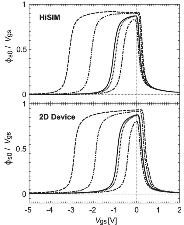
Fig. 3. Comparison of calculated derivatives of the surface potential at source side  $\phi_{s0}$  by HiSIM and a 2-D-device simulator. Bias conditions are the same as given in Fig. 2.
