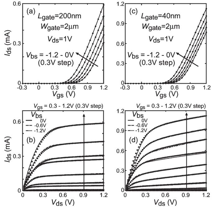
Fig. 10. Comparison of calculated  $I-V$  characteristics of a 40 nm CMOS technology with measurements for  $L_{gate} = 200$  nm (a)  $I_{ds}$  versus  $V_{gs}$  (b)  $I_{ds}$  versus  $V_{ds}$  and for  $L_{gate} = 40$  nm (c)  $I_{ds}$  versus  $V_{gs}$  (d)  $I_{ds}$  versus  $V_{ds}$ .
