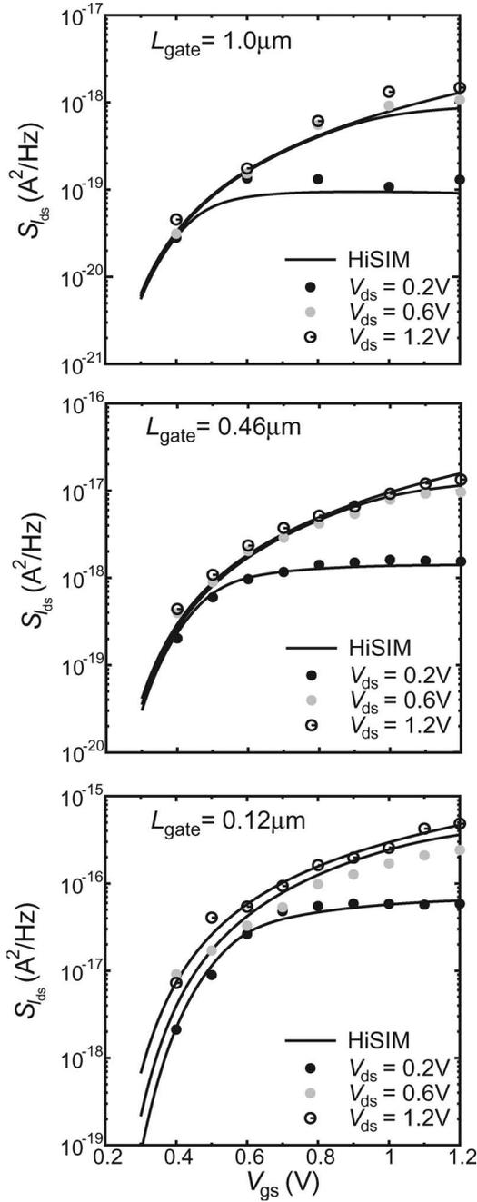
Fig. 12. Comparison of the bias dependence of measured and simulated drain current noise by HiSIM at a frequency of 100 Hz.
