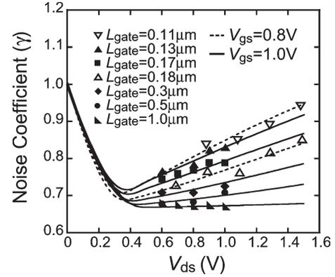
Fig. 13. Calculated noise coefficient  $\gamma$  with HiSIM as a function of drain voltage  $V_{ds}$  compared with measurements. Two different technologies are compared. For one technology measurements are represented by solid symbols and corresponding HiSIM results by solid lines, and for the other technology by open symbols and dashed lines.
