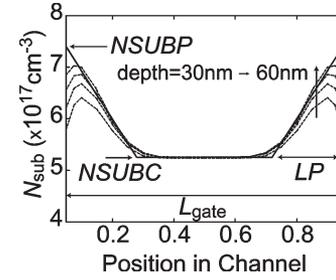
Fig. 5. Dashed curves are simulated impurity profiles by the 2-D-process simulator TSUPREM at various depths. The extracted pocket profile with the model is depicted by a solid line.
