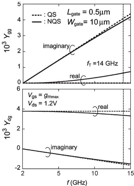
Fig. 16. Measured (open symbols) and calculated Y-parameters with the NQS model (solid lines) and the QS model (dashed lines) without the gate-resistance contribution.
