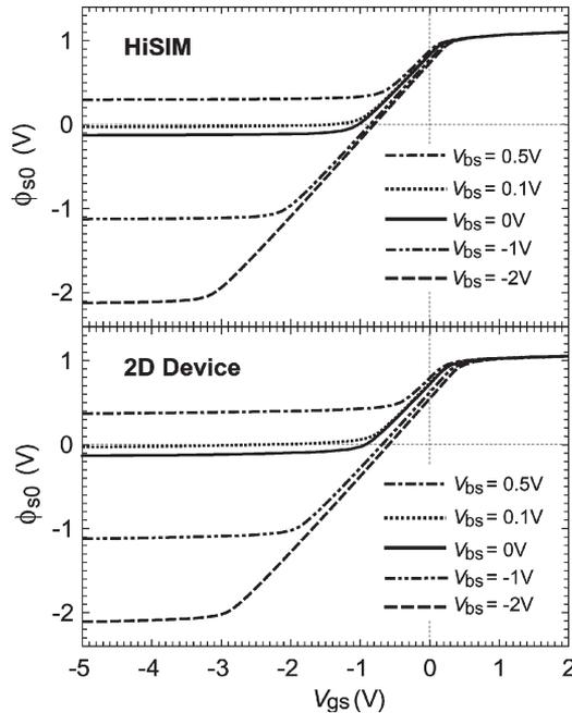
Fig. 2. Comparison of calculated surface potentials at source side  $\phi_{s0}$  by HiSIM and a 2-D-device simulator for various substrate voltages  $V_{bs}$  at drain voltage of  $V_{ds} = 0.1$  V. Gate length is fixed to  $2 \mu\text{m}$ .
