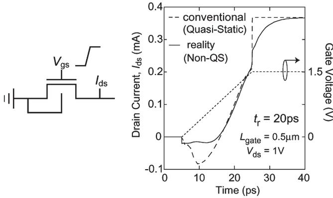
Fig. 14. Transient drain-current for 20-ps rising input. QS artifacts are eliminated with HiSIM's NQS model.
