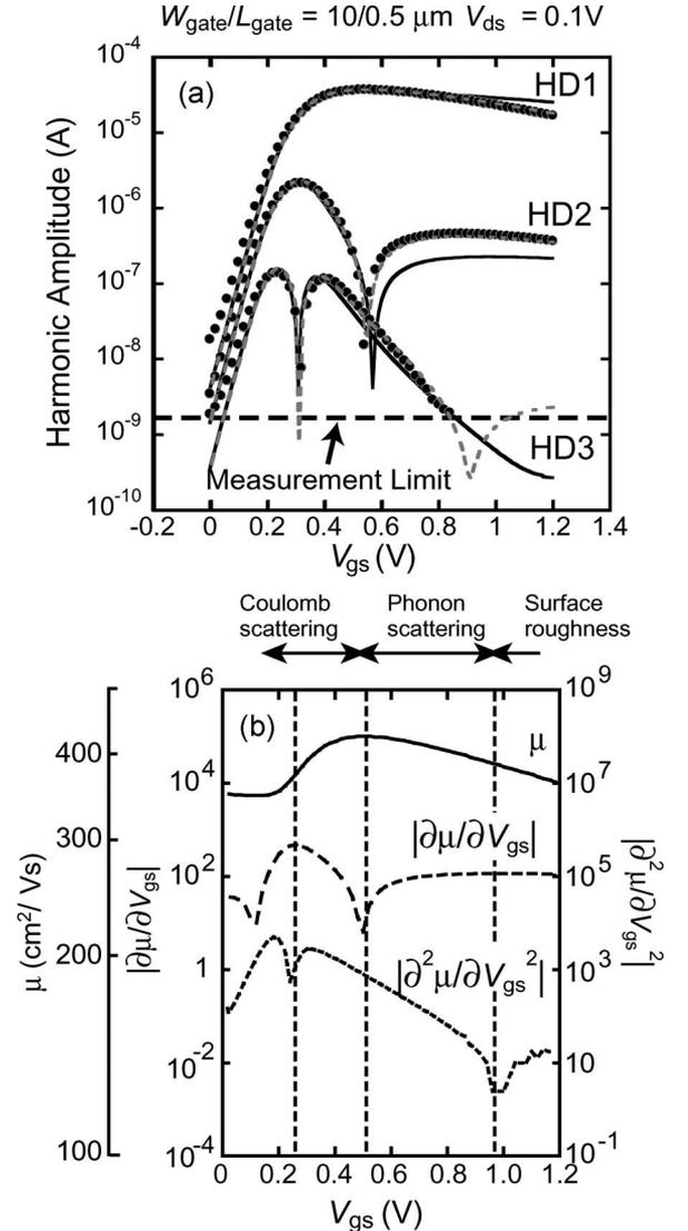
Fig. 11. (a) Simulated harmonic distortion characteristics at low drain bias and low frequency (1 kHz). (b) Mobility model of HiSIM and its derivatives. (Color version available online at <http://ieeexplore.ieee.org>.)
