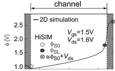
Fig. 1. Calculated surface potential by HiSIM at source side  $\phi_{S0}$  and at drain  $\phi_{SL}$  under the saturation condition. Simulated surface potential distribution along the channel with a 2-D simulator is also depicted for comparison. (Color version available online at <http://ieeexplore.ieee.org>.)
