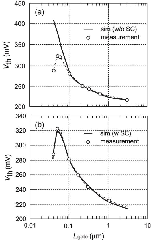
Fig. 7. Comparison of measurements and pocket-implant model for  $V_{th}$  as a function of  $L_{gate}$ . Results (a) with and (b) without SC are shown.
