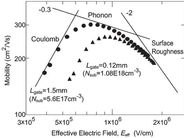
Fig. 9. Calculated mobility as a function of effective field for different MOSFET devices [29].
