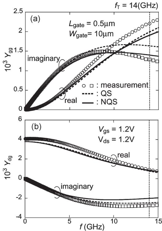
Fig. 15. Measured (open symbols) and calculated Y-parameters with the NQS model (solid lines) and the QS model (dashed lines). Model parameters are extracted by normal  $I$ - $V$  measurements and no fitting parameters are introduced. As external contribution only the gate resistance was included.
