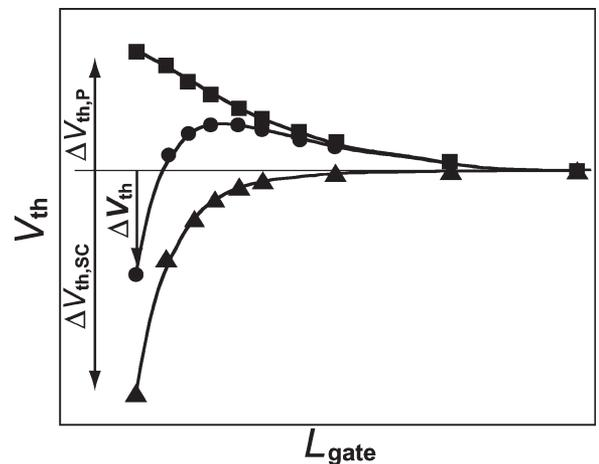
Fig. 4. Schematic plot of the separation of  $V_{th}$  into the contributions of the short-channel and the reverse-short-channel effect.
