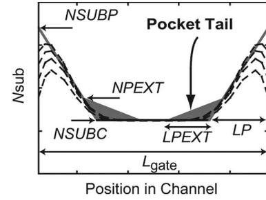
Fig. 8. Modeled pocket tail with NPEXT and LPEXT.
