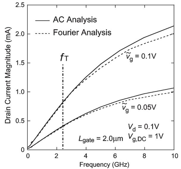
Fig. 17. Comparison of drain-current magnitude calculated with frequency-domain model and time-domain model.
