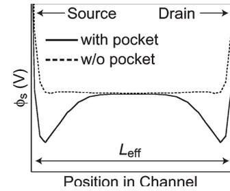
Fig. 6. Surface potential distribution along the channel simulated with a 2-D simulator.
