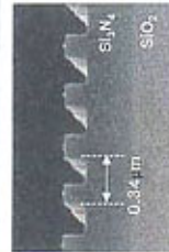
SEM Micrograph of the Fabricated Grating Coupler (Cross Section)
