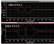
**•**Voltage Gain after LNA 2 = 15.6dB for Gaussian monocycle (center frequency = 5GHz, 3dB bandwidth=5.8GHz)
