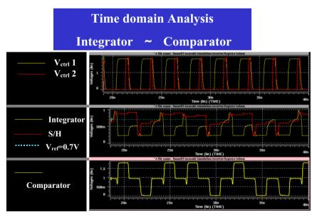
•Analog signal is converted to digital signal after integrator – comparator.
