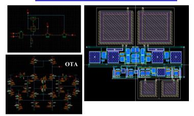
Integration time = 1.25ns (half of chip rate)Comparator: Inverter chopper type Comparator
