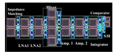
•TSMC 0.18μm rule (*V<sub>dd</sub>*=1.8V) •Differential implementation
