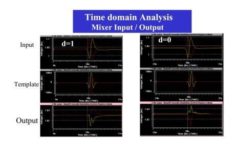
Succeed to demodulate data from the pulse position modulated signal using second derivative Gaussian template.
