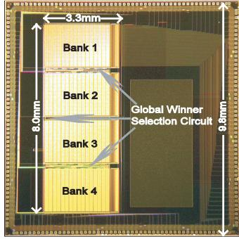
Figure 3: Chip photo of the 4-bank associative-memory (0.35um CMOS).
