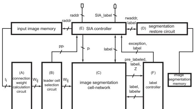
Figure 7: Block diagram of the cell-network-based image segmentation architecture with subdivided-image approach (SIA).
