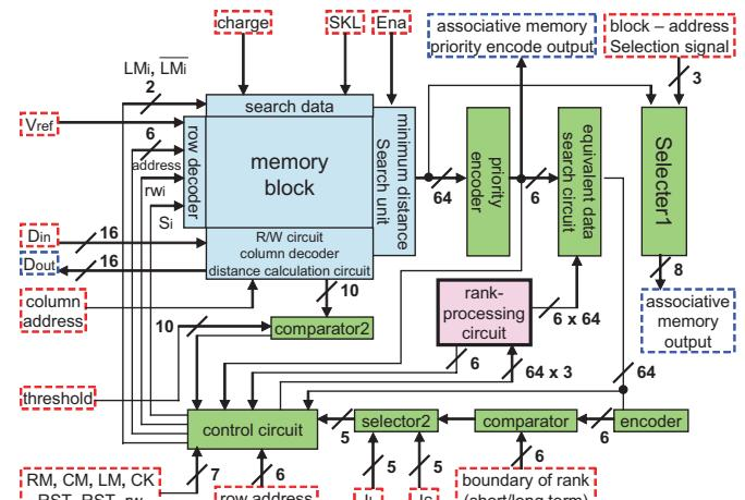
Figure 6: Associative-memory-based automatic pattern learning architecture with 64 patterns. Long/short-term-memory size, parameters  $J_L$ ,  $J_s$  and the threshold in the algorithm can be set externally.
