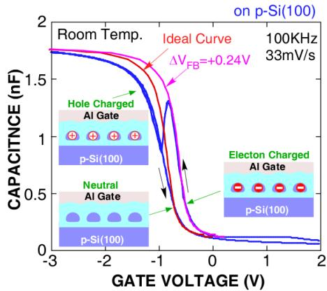
**C-V & I-V Characteristics of Si-QDs Floating Gate MOS Capacitors Fabricated on p-Si(100) & n-Si(100)**
