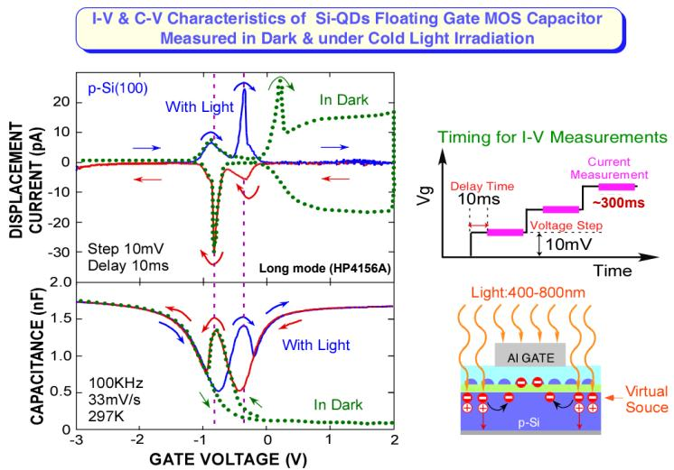
**I-V & C-V Characteristics of Si-QDs Floating Gate MOS Capacitor Measured in Dark & under Cold Light Irradiation — Light Intensity Dependence —**
