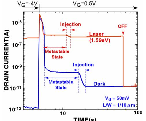
Fig. 2 Temporal changes in the drain current measured at  $V_g = 0.5V$  under irradiation of 780nm (1.59eV) light and dark condition after complete discharging of the Si-QDs floating gate at  $V_g = -4V$ .
