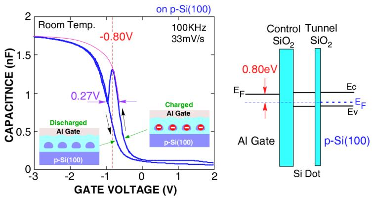
**Comparison between Measured and Simulated C-V Curves for Si-QDs Floating Gate MOS Capacitor**
