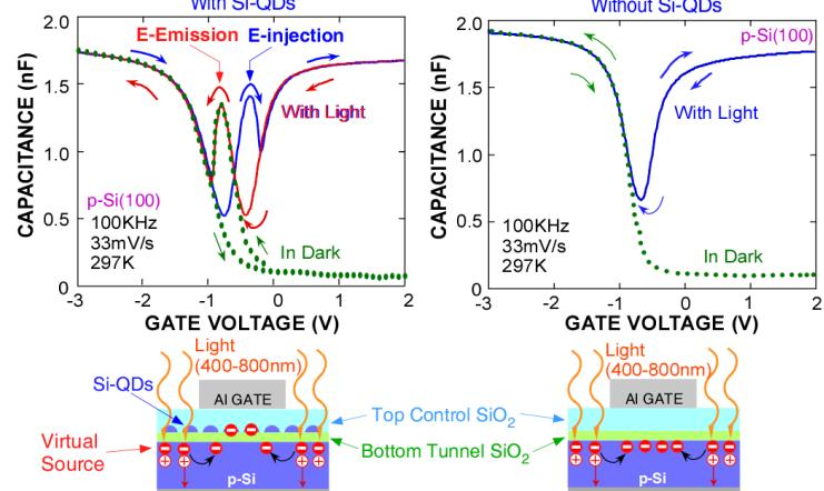
**I-V & C-V Characteristics of Si-QDs Floating Gate MOS Capacitor Measured in Dark & under Cold Light Irradiation**
