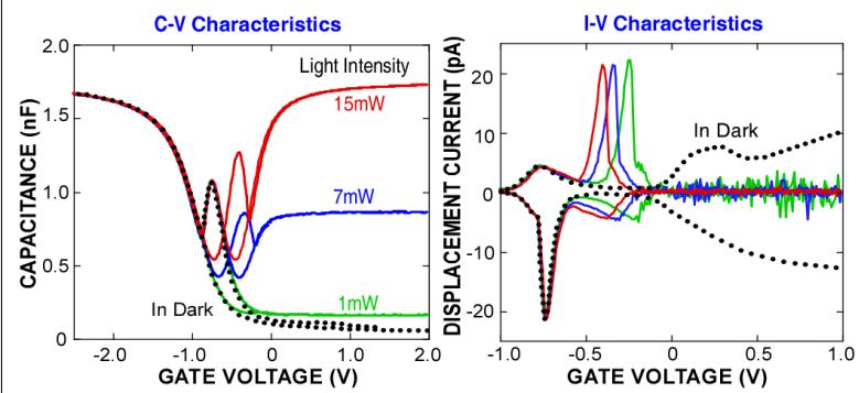
**I-V & C-V Characteristics of Si-QDs Floating Gate MOS Capacitor Measured in Dark & under Cold Light Irradiation**
