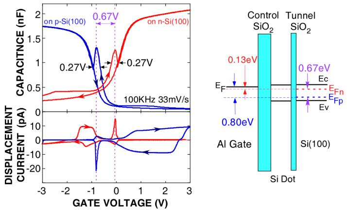
**C-V Characteristics of MOS Capacitors with & w/o Si-QDs Floating Gate Measured in Dark and under Cold Light Irradiation**
