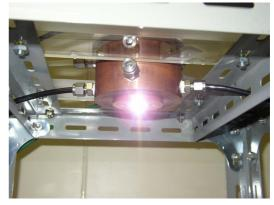
Fig. 1. Photograph of plasma jet generated by a DC arc discharge under atmospheric pressure.
