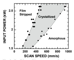
Fig. 3. Conditions of input power to the plasma source and scanning speed for the crystallization of a-Si films.
