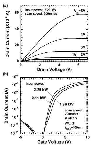
Fig. 4. Output (a) and Transfer (b) characteristics of TFTs fabricated with PJC Si films.
