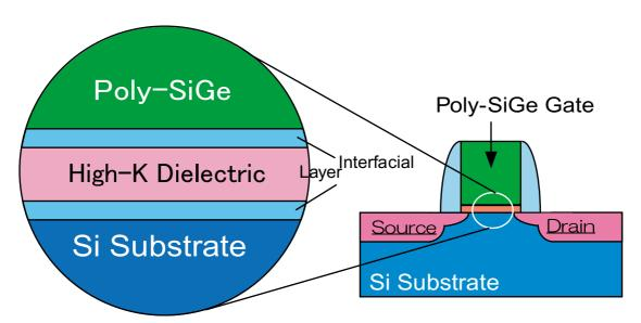
Cross-sectional view of MOS transister and gate electrode(Poly-SiGe)/high-k stacked structure. An interfacial layer was formed at high-k/electrode and high-k Si substrate interface. Therefore, expected perfomance improvement cannot be obtained. It's need to supress the growth of interfacial layer.
