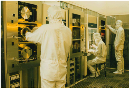
熱酸化及び減圧CVD装置 Oxidation furnaces and low-pressure CVD reactors.
