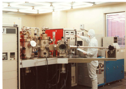
配線金属堆積用スパッタ装置 Sputtering system for metallization (Al, Ti, TiN).
